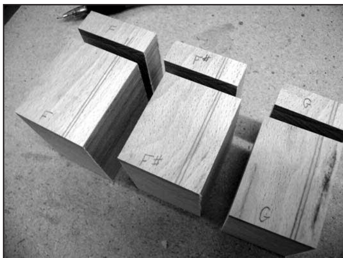
Figure 21. Spacer and block for each pipe.
