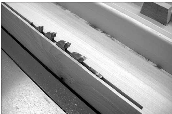
Figure 13. Block lumber is brought to oversize depth.
