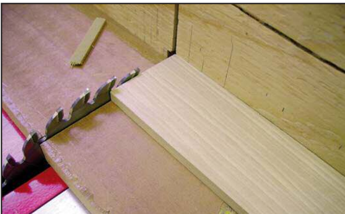
Figure 79. One end of front side is squared up on the table saw.
