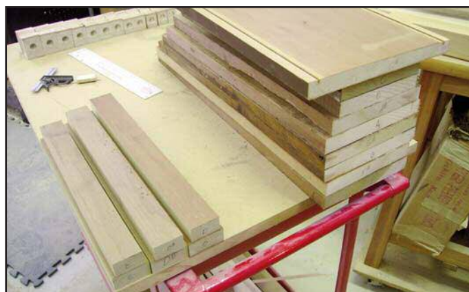
Figure 50. Side lumber grouped in pairs. Each piece will be resawn to create two sides.
