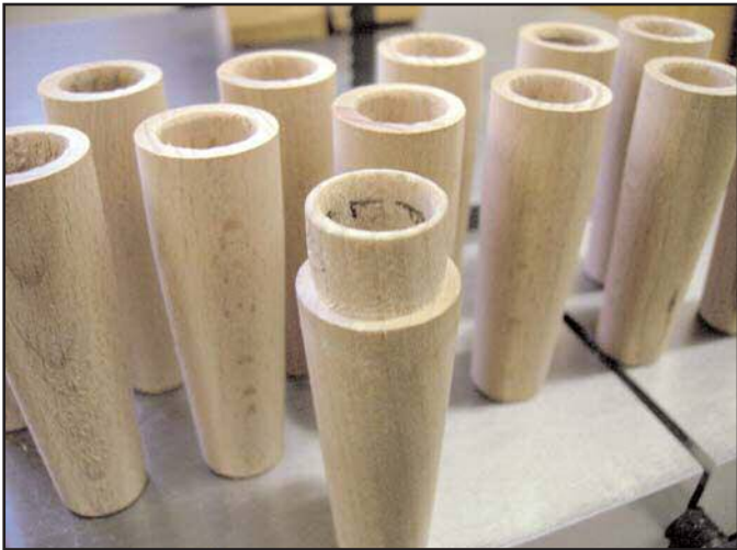
Figure 47. Tapers on all toes are completed. Sample toe is in front.
