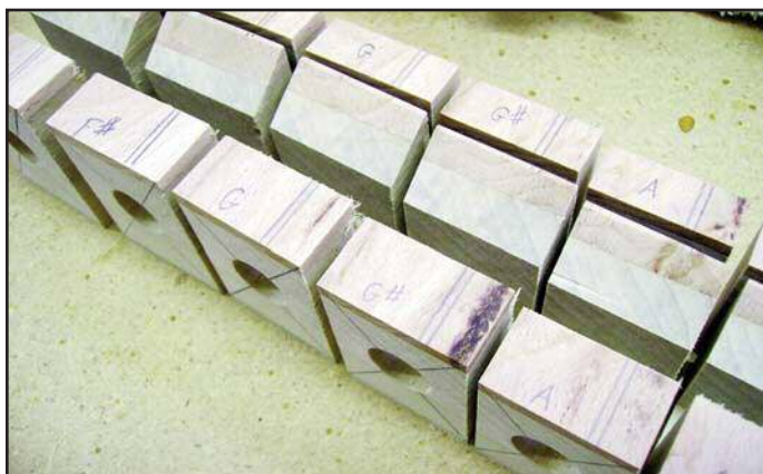
Figure 48. All cut-away areas removed from blocks.
