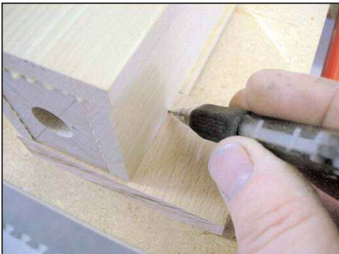
Figure 30. Marking pipe cap material for width.
