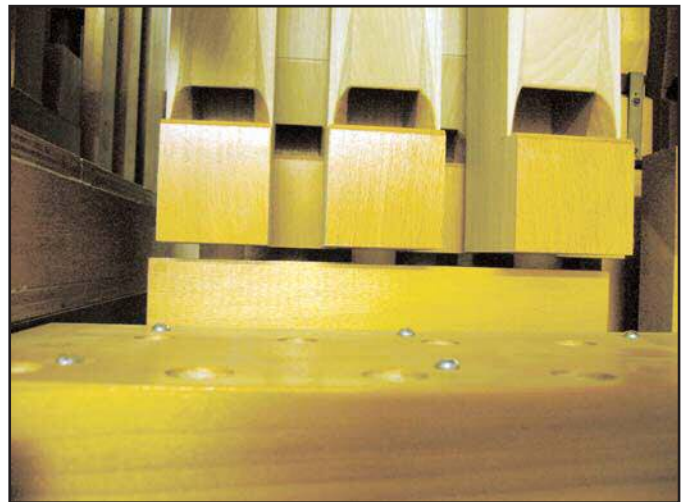
Figure 55 (above). Pipe body is checked for squareness with toe board and chest top.
