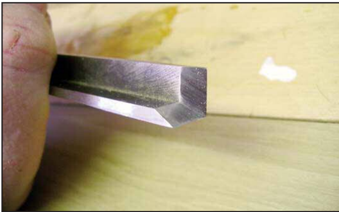
Figure 91 (below). Corners of chamfer more easily kept square with a corner chisel.
