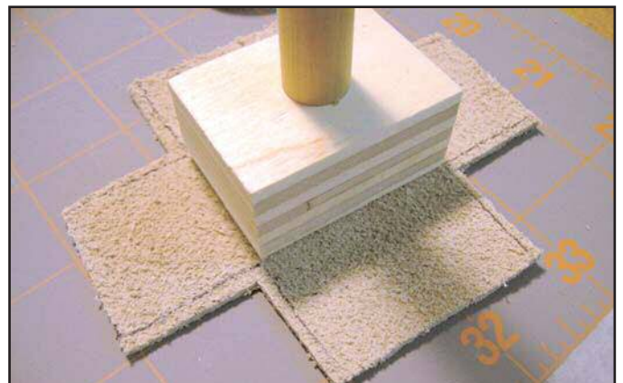
Figure 68. Leather is cut slightly larger than where lines are located.
