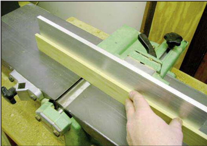
Figure 60 (above). One edge of each side piece is jointed.
