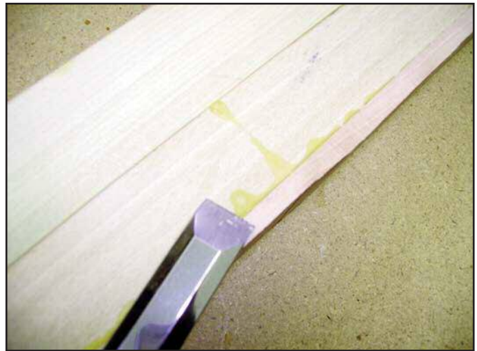
Figure 8. Remove excess glue with a chisel.
