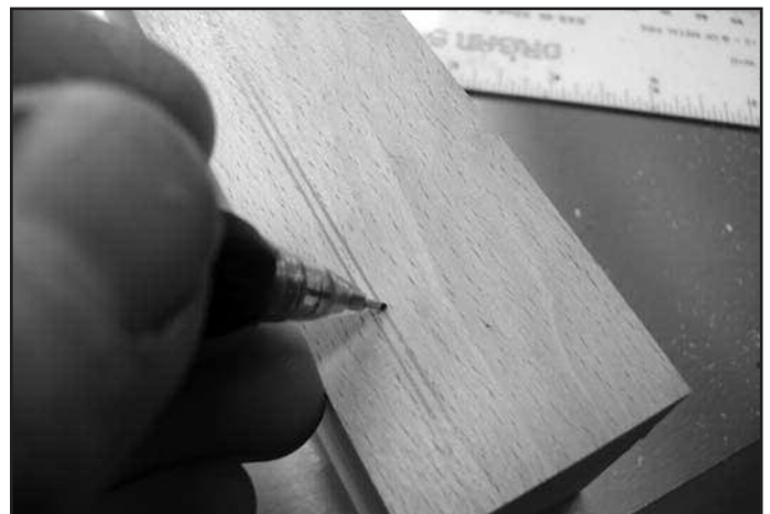
Figure 16. Reference lines are drawn on one side of block lumber.
