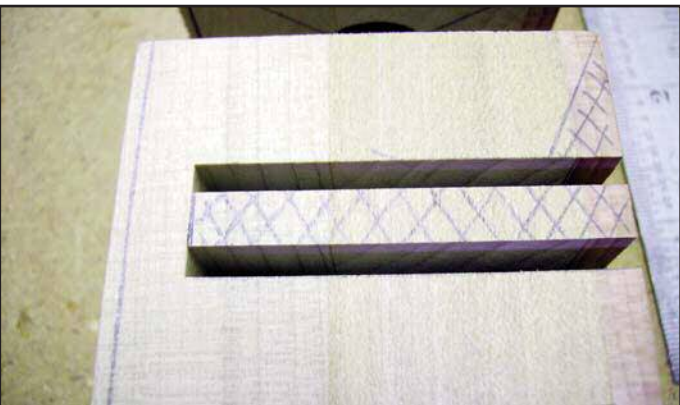
Figure 41. Top and bottom cuts completed on cut-away area.
