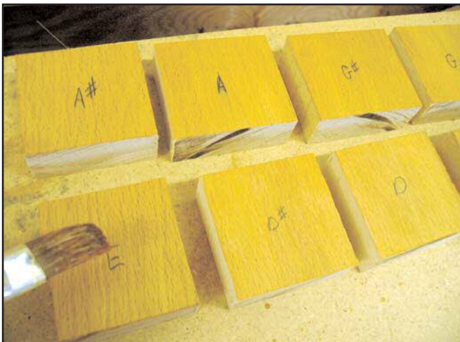
Figure 31. Inside of pipe caps with note names and shellac.
