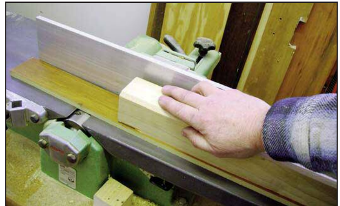
Figure 57. Inside face is machined flat on a jointer.
