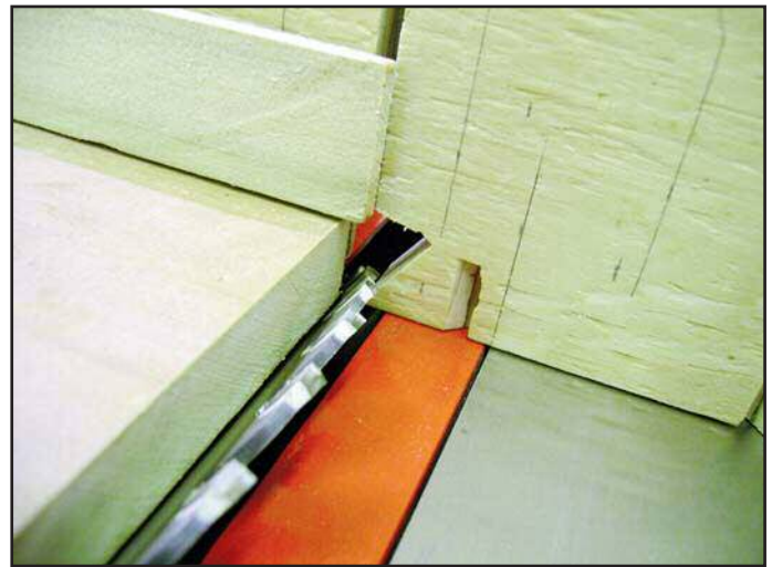
Figure 43. Be sure there is room for the cut piece to eject.
