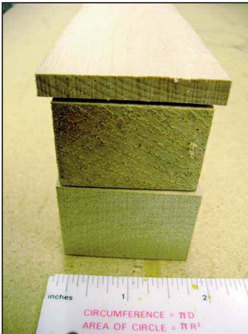
Figure 3. Three pieces of lumber are used to create the pipe blocks. The thin piece is a hardwood facing.
