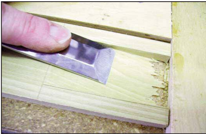
Figure 96. The chamfer will meet the cut-up mark on the backside, leaving a nice square window on the front of the pipe.
