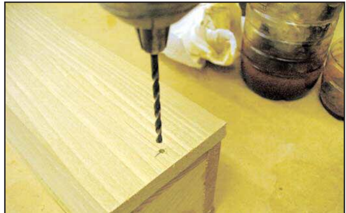
Figure 14 (above). Drilling for pipe front pin.
