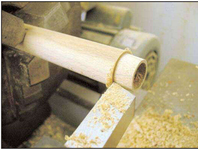
Figure 40. Taper of toe is machined.
