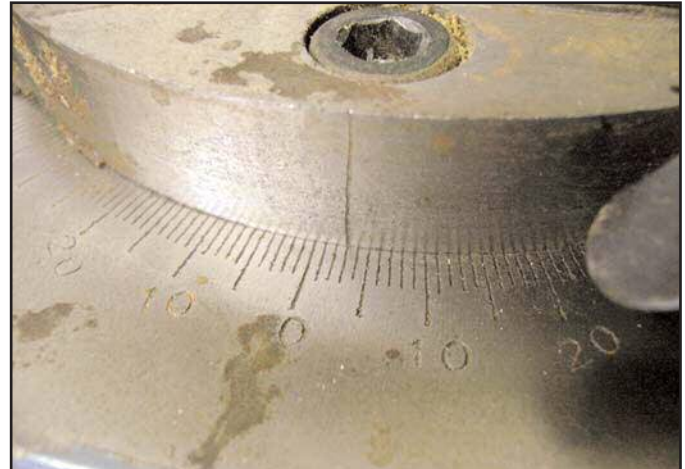
Figure 37. Compound slide of lathe is set to three degrees.
