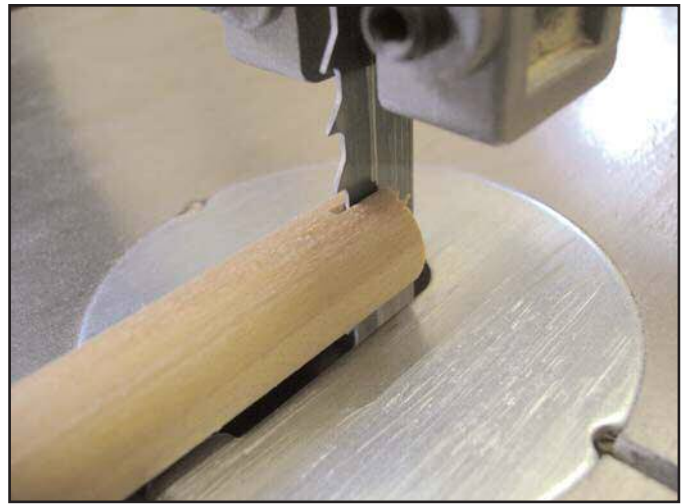
Figure 60 (above). Handle is split for wedge.
