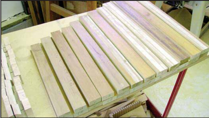
Figures 53 & 54. Note names are written on the end of each piece. All lumber is now rough cut.
