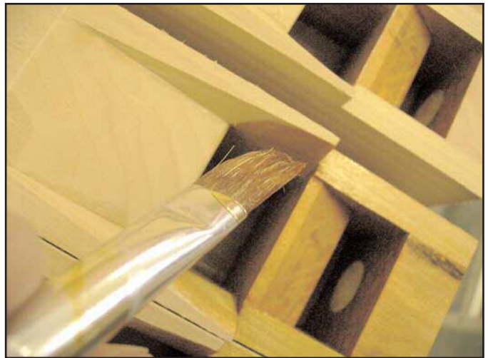
Figure 32. Shellacking area around windway.
