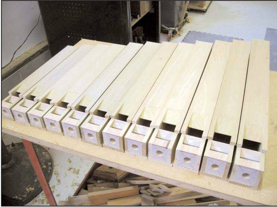
Figure 1. Nearly finished pipe fronts lying on pipe bodies.
