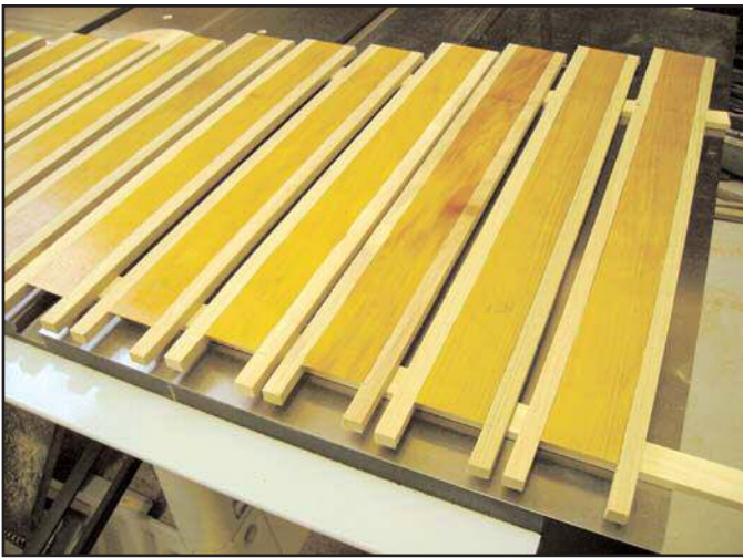
Figure 10. Pipe front insides all shellacked.
