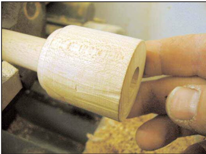
Figures 41 (above) & 42 (below). Gauge for checking taper of toe.
