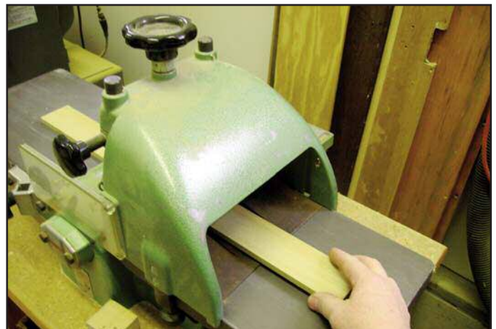
Figure 58. Other side is brought to finished thickness on a planer.
