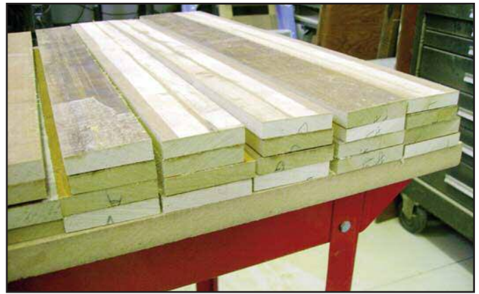
Figure 56. All side lumber is now resawn with four pieces for each pipe.
