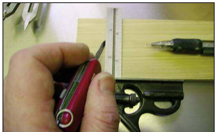
Figure 82. The top of the cut-up is marked on the inside of the front.
