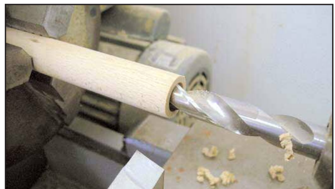
Figure 39. Toe hole is drilled.
