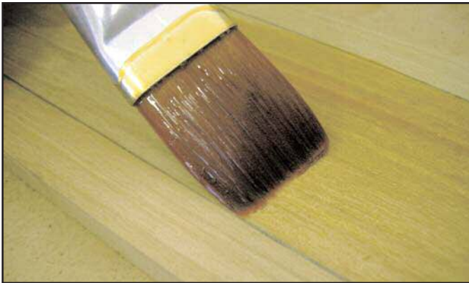
Figure 5. Shellac applied inside pipe front.
