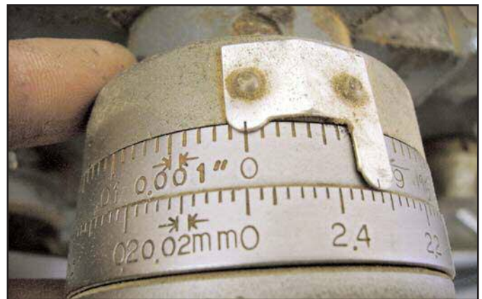
Figures 44. Hand wheel is zeroed so all toes are machined the same.
