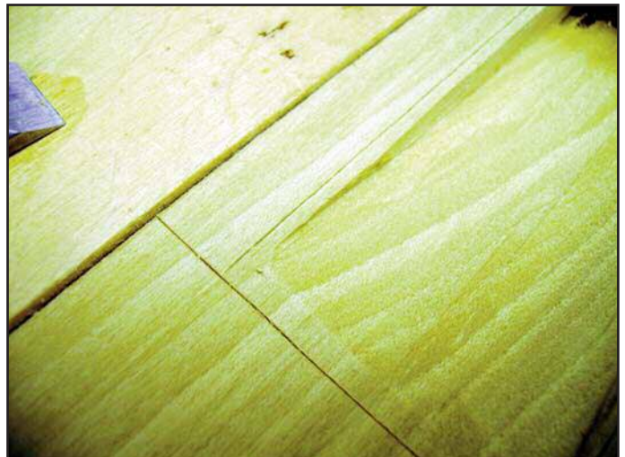
Figure 94 (below). Stay about one sixteenth of an inch away from the side mark until the chamfer is nearly finished.
