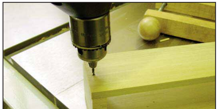
Figure 63 (above). Hole for the pin is drilled through side and into spacer.
