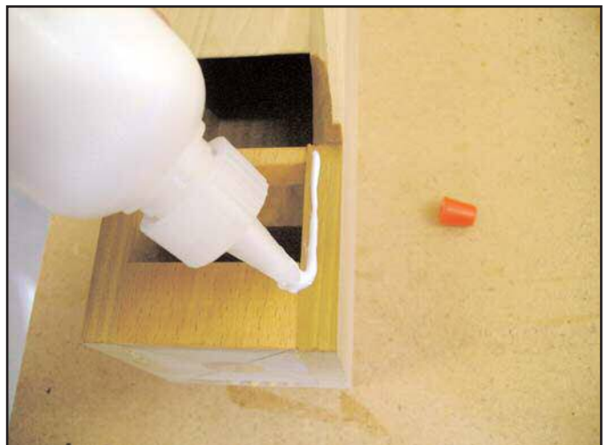
Figure 33. Gluing for pipe cap.
