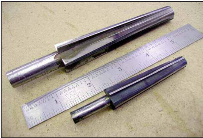
Figure 24. Tapered reamers for machining toe holes.
