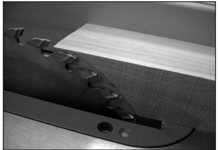
Figure 14. A minimum cut is made on hardwood face to assure flatness.
