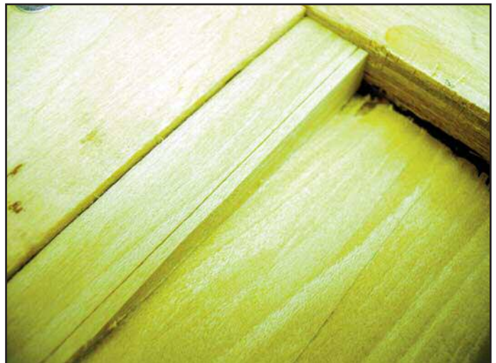
Figure 95. As the chamfer approaches the finished depth, it will meet with the backside.
