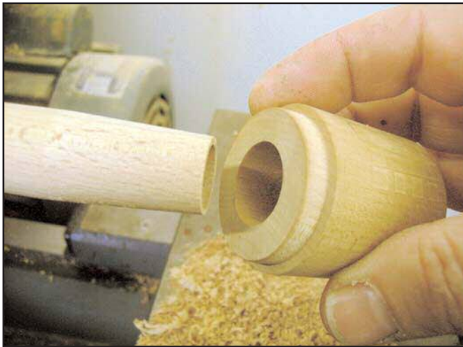
Figures 41 (above) & 42 (below). Gauge for checking taper of toe.
