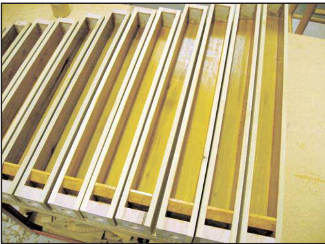
Figure 11. Pipe back and sides all shellacked inside.
